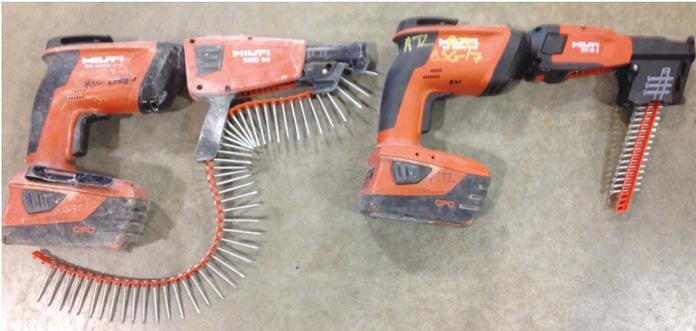
Reports have been positive on the new Hilti screw magazine (right) that are gradually being replaced in the field. The new magazine requires little adjustment when using different size screws.
